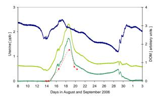
Figure 2. Dom signal removal from the uranine curve. From top to bottom: DOM curve, uncorrected uranine, corrected uranine, broken line: laboratory analysis of tracer for comparison.
