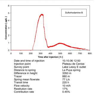
Figure 4. Tracer test at Lake of Lessy during low water.
