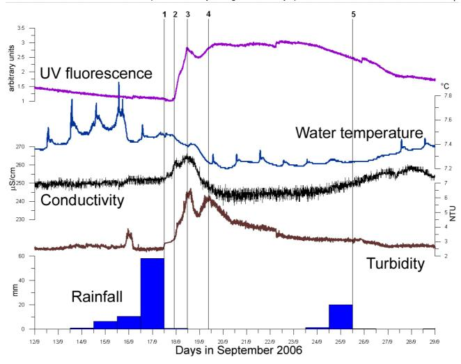
Figure 6. Series of typical events marked 1 to 5 during rise in the water level after rainfall. Daily spikes in water temperature is caused by poor isolation from the air. UV fluorescence results from dissolved organic matter (DOM). Rain height was recorded in the nearby valley of Grand Bornand
