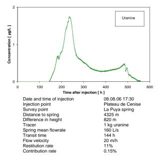
Figure 5. Tracer test at Plateau de Cenise.
