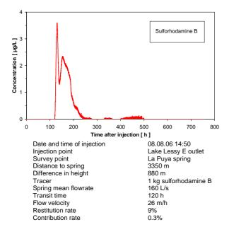
Figure 3. Tracer test at Lake of Lessy during high water.
