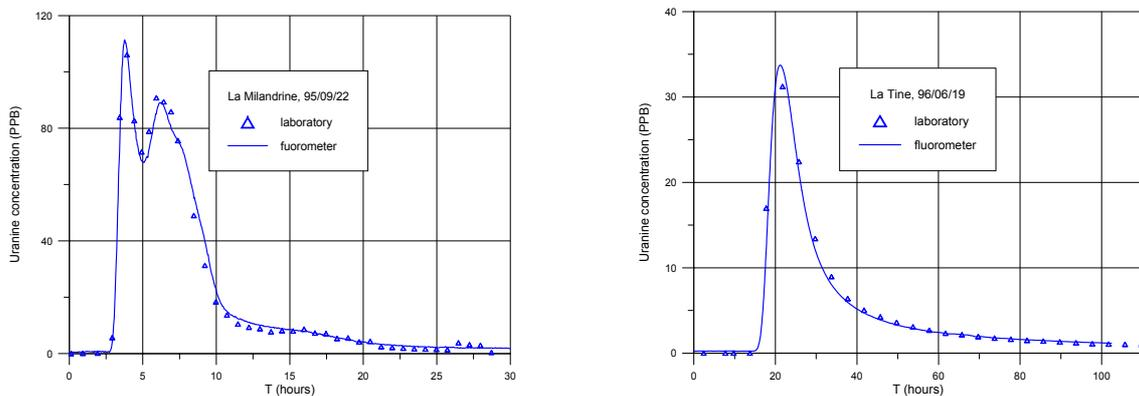
Fig. 2 a & b: Comparison of the results from the fluorometer (line) and the sampler (triangles) at 2 sites.
