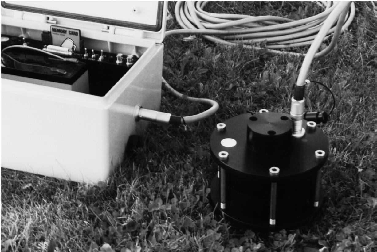
*Photo 1 : Fluorometer with its data acquisition box.*
