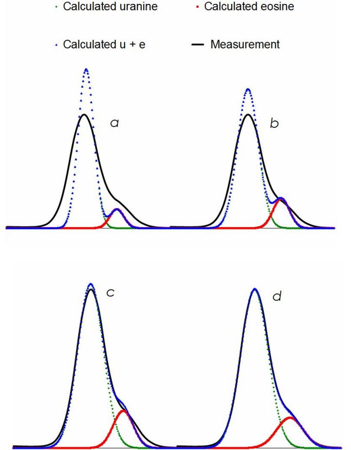
Figure 4. Separation of uranine and eosine from a 50-50% cocktail with the help of an optimization program based on the steepest descent in the space of the parameters. After 600 iterations, the calculated curve matches the measured one. a to d: 100, 200, 400 and 600 iterations. Horizontal axis: wavelength.
