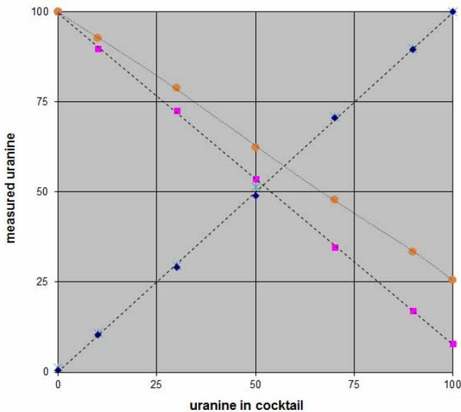
Figure 5. Measured vs. actual uranine and eosine concentrations in a cocktail. Results from the Perkin-Elmer spectrofluorometer and separation by fitting of two Gaussian curves. For comparison, the circles represent the result of the separation by the method of Wernli (2005).
