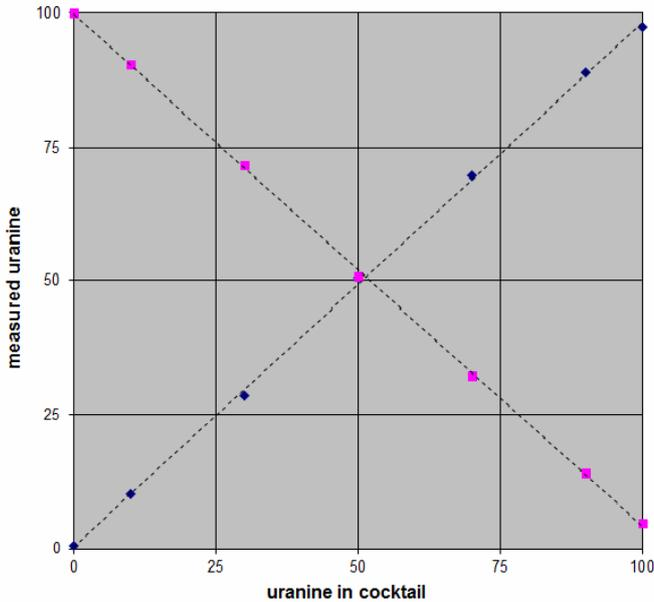
Figure 3. Measured vs. actual uranine and eosine concentrations in a cocktail. Results from the flow-through field fluorometer as obtained by solving Equation 1.
