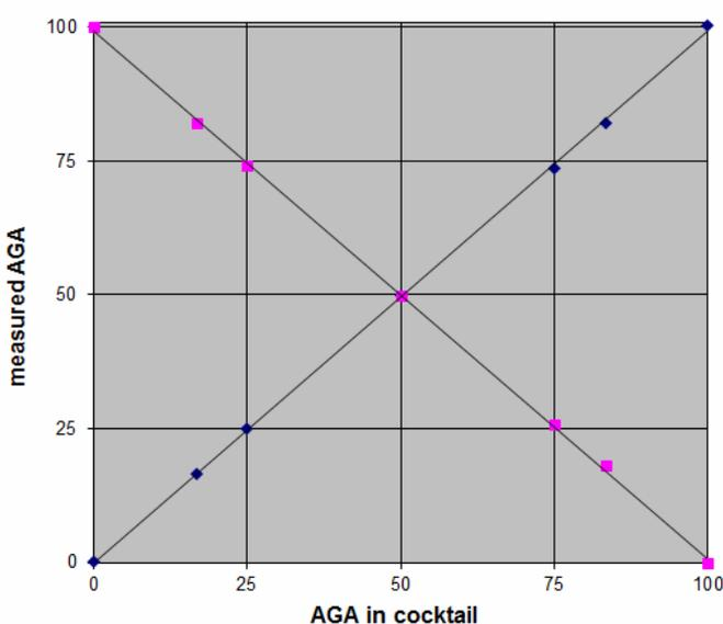
Figure 6. Measured vs. actual AGA and naphthionate concentrations in a cocktail. Results from the flow-through field fluorometer as obtained by solving Equation 1.
