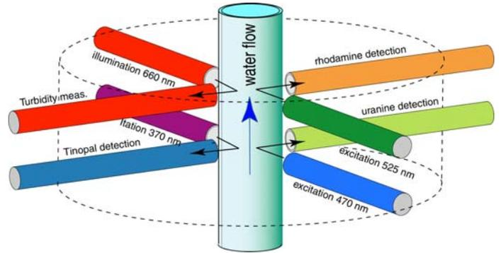
Figure 2. Setup of the flow-through field fluorometer.
